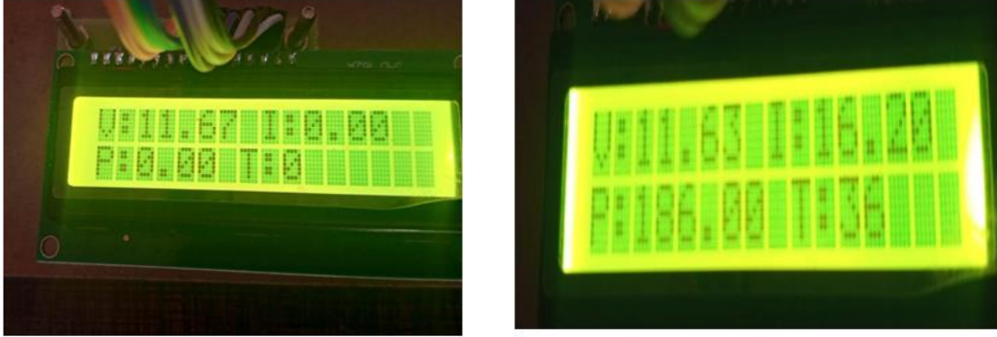
Figure 3: Shows the V, I, P ,T with and without Loads
