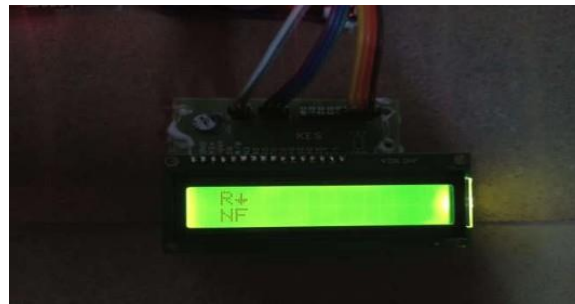
Fig. 7. No Fault Indication
