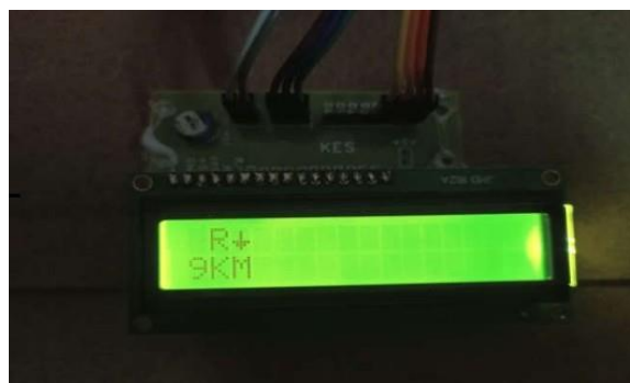
Fig. 8. Fault Indication at 9 km Distance
